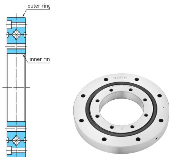
6. Customized type (CRBX): The bearing could be designed and modified in accordance with the requirements of customer with more innovative structure. The surface treatment could also be conducted in accordance with the environmental requirements of customer.
