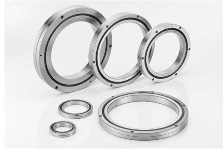
2. Split inner ring type (CRBB): Consisted of two inner semi-rings and an outer ring, which is suitable for rotating of outer ring.
